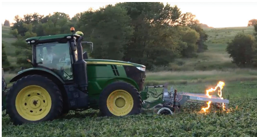
POWER PLAY. With a focus on growing cover crops to help reduce levels of atmospheric CO 2 , Keota, Iowa, organic farmer Levi Lyle uses alternative weed control technologies, such as zapping them with electricity.
